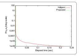
We set  $\alpha := 1$ ,  $\mu := 1/10^5$ ,  $\alpha_n := 1/(n+1)$   $(n \in \mathbb{N})$ , and  $\beta_n := 1/(n+1)^2$   $(n \in \mathbb{N})$  in Algorithm 3.1 and compared Algorithm 3.1 with the Halpern algorithm (1) with  $\alpha_n := \mu/(n+1)$   $(n \in \mathbb{N})$ . In the experiment, we set  $C_i$  (i = 0, 1, ..., m) as a closed ball with center  $c_i \in \mathbb{R}^N$  and radius  $r_i > 0$ . Thus,  $P_i$  (i = 0, 1, ..., m) can be computed with
